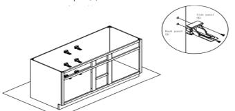
Step 10: Insert drawer slide runner to the rear slide bracket and screw the drawer slide to the guide hole of front frame (A) and hole for drawer slide.
