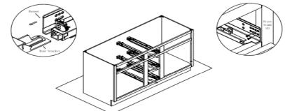
Step 11: Put the drawer box on the drawer slide and push the drawer box to make the end | Step 12: Install door panel (G). Screw the hinge to of runner is lock to the hole of the drawer back panel. Complete the installation of the drawer box when your hear sound click which mean the locking device is locked on the drawer slide.
