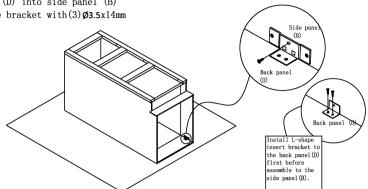
Step 8: Install corner block. Install rainbow bracket to the side panel (B), front frame (A) and back panel (D) with the (4) Ø3.5x16mm screw.
