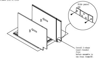
Step 3: Install bottom panel. Insert the bottom panel (C) into groove of side panel(B) until it into the groove of front frame(A).
