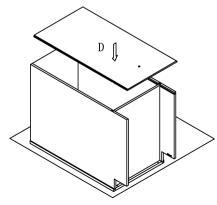
Step 5 : Install screw(5) Ø3.5x35mm into back panel (D).
