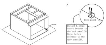
Step 8: Install corner block. Install rainbow bracket to the side panel (B), front frame (A) and back panel (D)with the (5)Ø4\*16mm screw.
