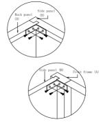
Step 9: Install the drawer slide rear bracket. Screw the rear slide bracket to the back panel (D)
