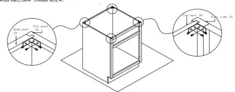
Step 9: Install door panel (G). Screw the hinge to the front frame (A) and door (G).
