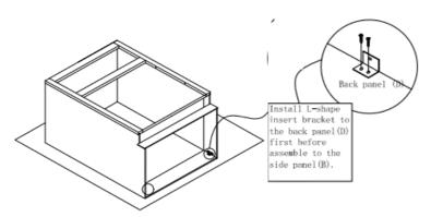
Step 8: Install corner block. Install rainbow bracket to the side panel (B), front frame (A) and back panel (D)with the(5)Ø4\*16mm screw.
