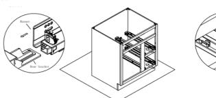
Step 11: Put the drawer box on the drawer slide and push the drawer box to make the end of runner is lock to the hole of the drawer back panel. Complete the installation of the drawer box when your hear sound click which mean the locking device is locked on the drawer slide.
